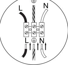
Expanded Wiring Diagram
