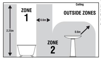
This product is suitable for use in Zone 2 and outside Zones of a bathroom. See diagram. If this unit is being fitted in a room containing a bath or shower, a 30mA RCD must be used, in accordance with IEE regulations.
