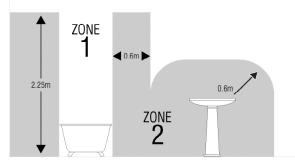
This product is suitable for use in Zbn 2 and outside Zones of a bathroom. See diagram. If this unit is being fitted in a room containing a bath or shower, a 30mA RCD must be used, in accordance with IEE regulations.
