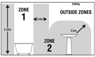
2 and outside Zones of a bathroom. See diagram. If this unit is being fitted in a room containing a bath or shower, a 30mA RCD must be used, in accordance with IEE regulations.
