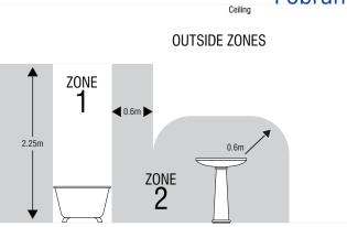
This product is suitable for use in Zo 2 and outside Zones of a bathroom. See diagram.
