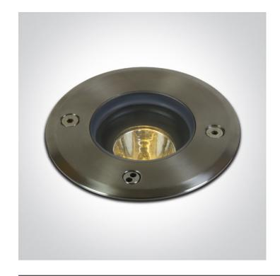
3W COB LED inground uplight with a 5° beam which is tiltable +/-20°. IP67, stainless steel 316L and die cast aluminium body.
