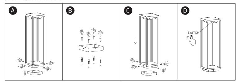
LED 100% when movement detected. LED 15% when no movement detected.
