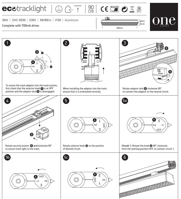
Circuit 3: Rotate the knob 🔕 180° clockwise
