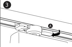
Rotate tab clockwise 90° to connect the adaptor to the neutral circuit.
