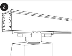
Ensure the track adaptor is inserted with the correct orientation.
