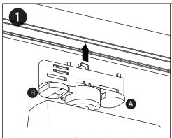
To mount the track adaptor into the track system, check that both tabs (A) (B) on the adaptor are in the "open" position and insert into the track.
