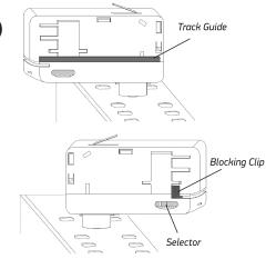
Before plugging the adaptor in the track line, make sure that the selector is on position 0 and the blocking clip is out as shown.
