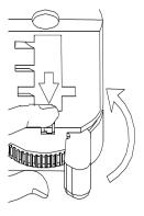
Once the adaptor is plugged in, pull the clip in central position as shown. This will safely block the adaptor in the track line.
