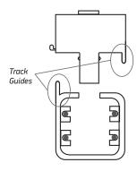
When plugging the adaptor in the track line make sure to respect the guide lines on both the adaptor and the track line, unproper connection would cause a short circuit.
