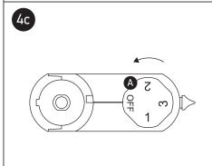
Circuit 3: Rotate the knob (A) 180° clockwise from the starting position OFF, to connect circuit 3.
