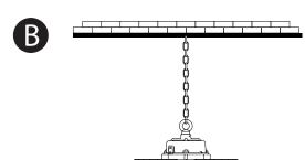
Use a chain, cable, mounting hook, or other mounting hardware to suspend the luminaire. Make sure the mounting hardware is securely attached to a stationary structure and strong enough to safely suspend the luminaire.
