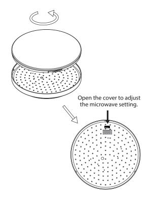
By selecting the combination on the DIP switch, sensor data can be precisely set for each specific application.
