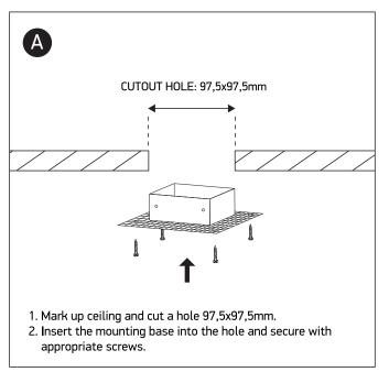
100-240V | MR16 | GU10 | 10W | IP20 | Die cast | Trimless | Adjustable
