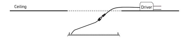
C Install fitting using springs supplied.
