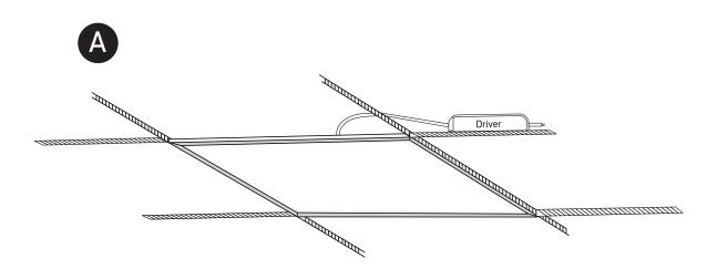
Recessed fitting for 620x620mm T-rail false ceilings.
