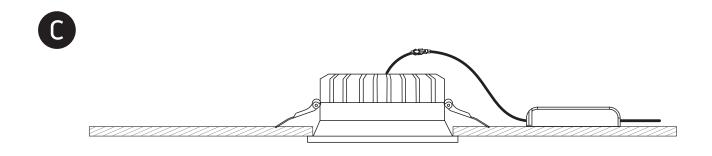
\*IP54 is the protection degree of the fitting under the ceiling. The fitting part hidden in the ceiling is IP20
