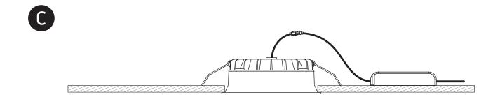
\*IP54 is the protection degree of the fitting under the ceiling. The fitting part hidden in the ceiling is IP20
