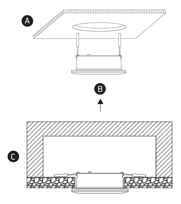
\*IP65 is the protection degree for the visible part of the fitting under the ceiling. The part of the fitting hidden in the ceiling is IP20.
