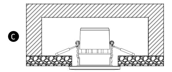
\*IP65 is the protection degree for the visible part of the fitting under the ceiling. The part of the fitting hidden in the ceiling is IP20.
