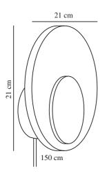
Voltage (V): 220-240 Volt IP degree: IP20 Class (Class 1, Class 2, Class 3): Class 2 (Double isolated) Socket type: LED Module Switch placement: On the cable Parallel connection: False
