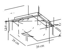
Voltage (V): 220-240 Volt IP degree: IP44 Maximum bulb wattage (W): 15W
