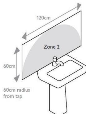
THIS LIGHT FITTING IS IP44 MAKING IT SUITABLE FOR ZONES 1 AND 2
