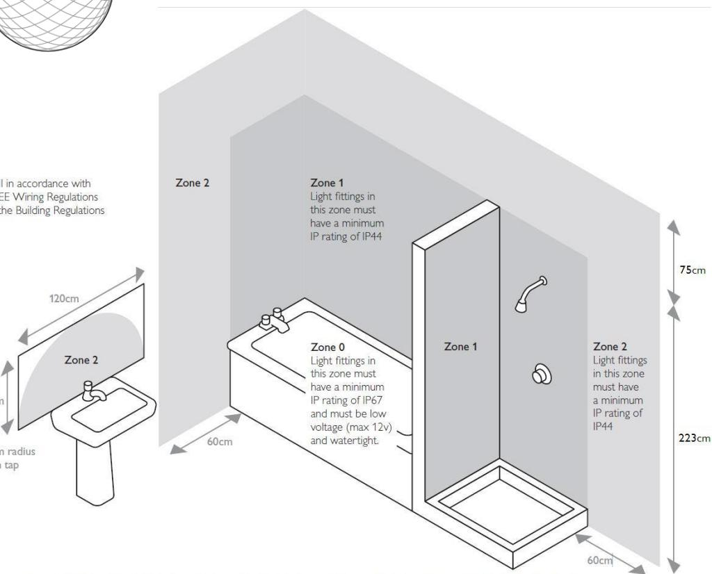
THIS LIGHT FITTING IS IP44 MAKING IT SUITABLE FOR ZONES 1 AND 2
