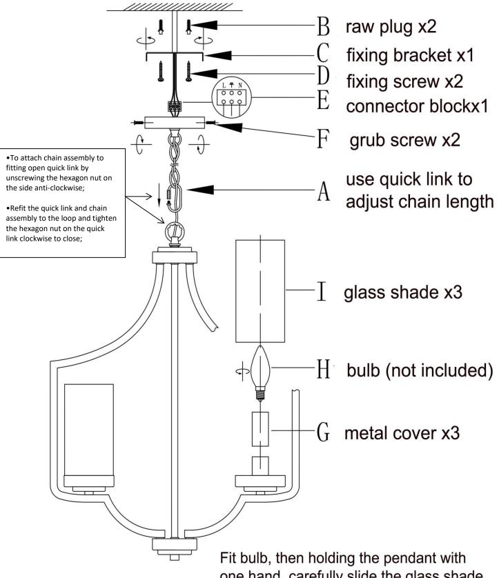
one hand, carefully slide the glass shade over the bulb and lamp holder assembly. To fit and change light bulb, carefully remove glass shade.
