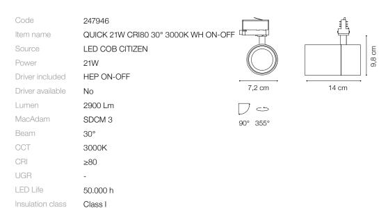
Extruded aluminum cylindrical tracklight suitable for installation on three-phase track. White or black powder coating, 355° turning head and 90° adjustable, the power driver is included and located in the cylindrical body of the projector itself. Dimmable 1-10 or DALI version available, Light source with integrated
