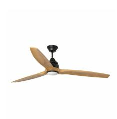
ALO L is a ceiling fan with light ideal for the ventilation of rooms up to 17'6m2. Made from metal, blades from wood and opal glass difusser. Operated on remote control (included). This ceiling fan has reverse function and it is suitable for inclining room. It has 3 adjustable speed with a 14 - 30 - 56W and 80 - 113 - 155 revolutions per minute depending on speed. Airflow: 129.29 m3 min / 4564 CFM.
