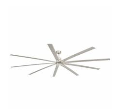
Ceiling fan with light extra large from 28m2. Operated by remote control (included) setted up with 6 dimmable speeds 15 - 20 - 25 - 30 - 35 - 56W and 50 - 55 - 60 - 65 - 70 - 78rpm. MANHATTAN has winter / summer function and it is suitable for inclining roof. Airflow: 269,12 m3 min / 9500 CFM.
