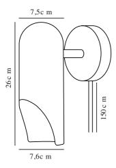
Voltage (V): 220-240 Volt IP degree: IP20 Maximum bulb wattage (W): 8W Class (Class 1, Class 2, Class 3): Class 2 (Double isolated) Socket type: GU10 Switch placement: On the base Parallel connection: False
